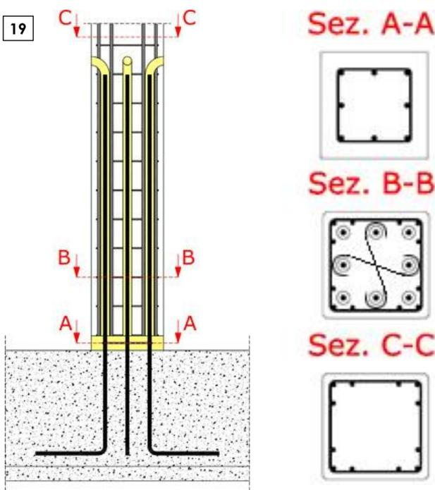
Fig. 19 – Connection to the foundation with protruding bars and sheaths.
