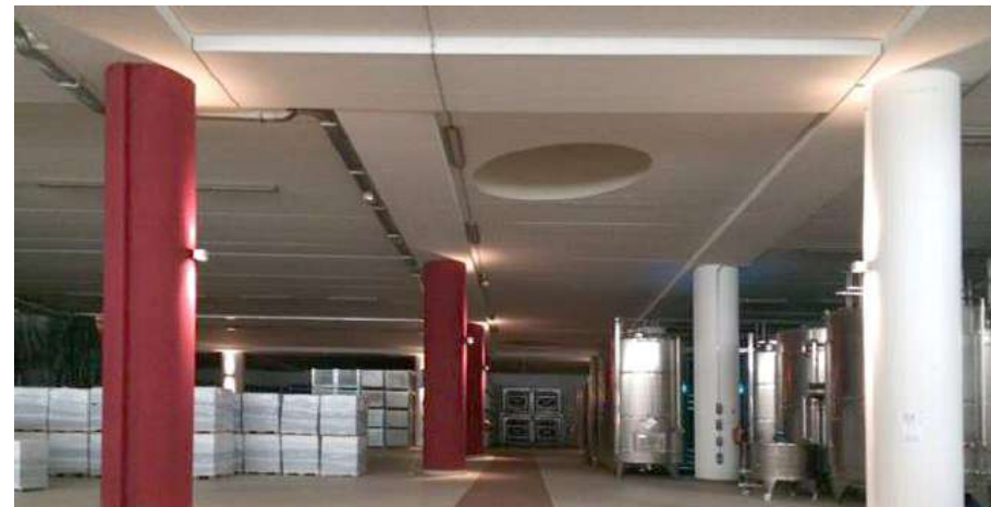
Azienda Agricola (BS): Travi PREM a2 – Solai a Lastre alveolari – Pilastri in c.a. in opera.
